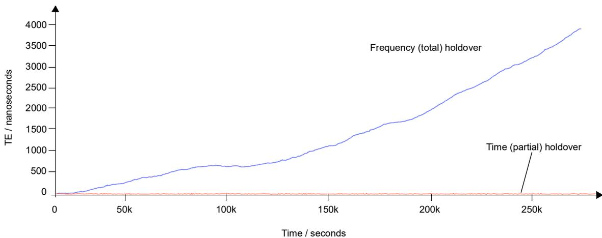
**Figure 4** Frequency and time holdover performance for a holdover period of three days.
