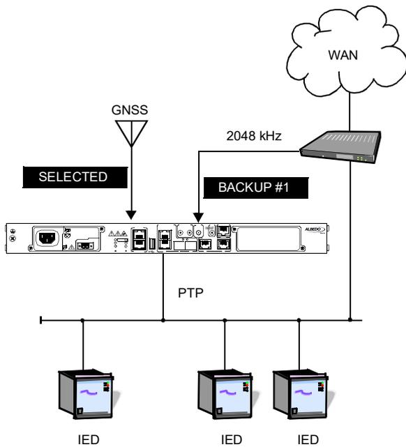
**Figure 1** Using a frequency backup. The backup clock reference is derived from the WAN.
