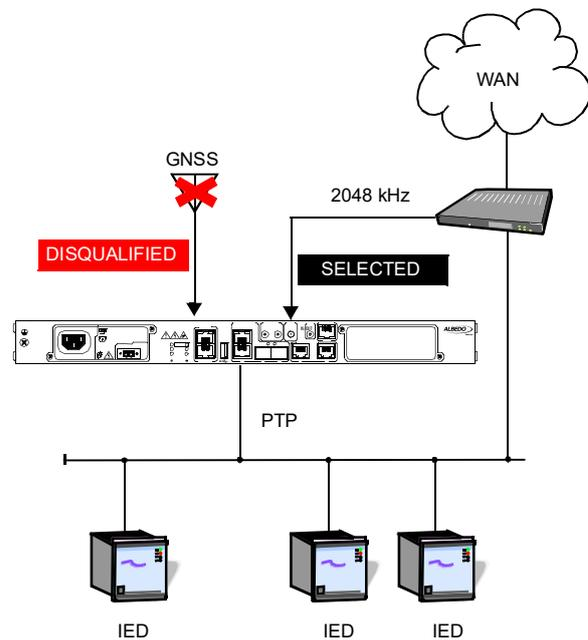
**Figure 2** If the main reference is lost, the backup is selected.
