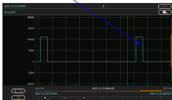
Figure 9 Test results obtained when the interlink port of a redbox is loaded by variable traffic and measured at LAN A and LAN B (only LAN A results are shown). The received traffic has a ramp shape. If the traffic load exceeds certain limits, the DUT starts dropping packets.
